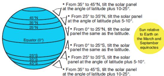
You also may wish to adjust the tilt closer to horizontal in summer and closer to vertical in winter. Please note that build-up of material (e.g. dust or bird droppings), or shading (e.g. from trees or buildings) will have an impact on the power output of the panels.
